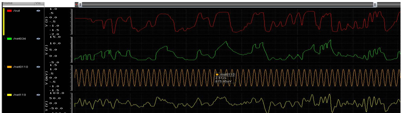
FIG. 10. FREQUENCY RESPONSE OF SCF SECOND ORDER BPF WITH INPUT EEG SIGNAL.
